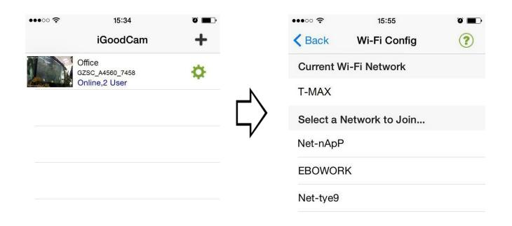
Choose a target Wi-Fi Network and input password, and then disconnect net cable when the camera starts initialization. After initialized, the camera will switch to Wi-Fi connection in 60 seconds.
